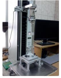
Fig. 1. Testing machine Zwick BDO-FB0.5TH with mounted "back-extrusion cell" device
